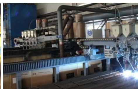
SUBMERGED ARC LINE
